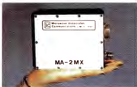
Dimensions: 4 3/4" x 2 1/2" x 5 3/4", Weight: 3.53 lbs. Power output 12 watts, high stability 21-channel synthesizer, internal VSWR and thermal protection, dual audio channels.
